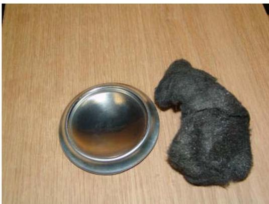
The first step is to use fine steel wool - or a scouring pad. This will remove any printing that is on the bottom and will get rid of any larger scratches or matt finishes.
