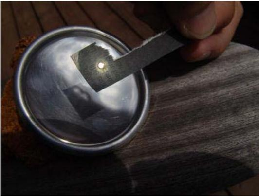
.... until the focal point is reached - at which point the paper will probably burn through - as in this photo. Note the position of this focal point -and place your other tinders in the same place.
