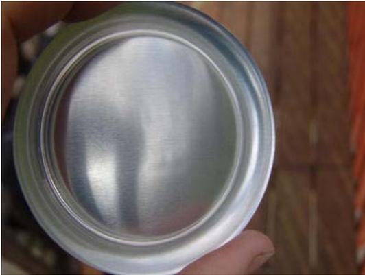
For comparison, this is the back-side of the can bottom. This shows what the original surface looked like.
