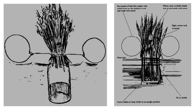
Duck Trap: These traps are floating snares, that use a bottle as the float, and grain as the bait.
