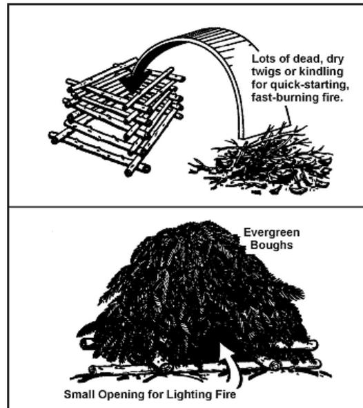
**Figure 19-2. Smoke Generator—Ground**
