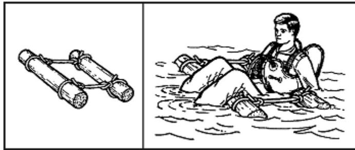
**Figure 17-8. Log Flotation**
