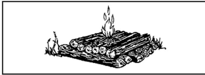
**Figure 7-3. Base for Fire in Snow-covered Area**
